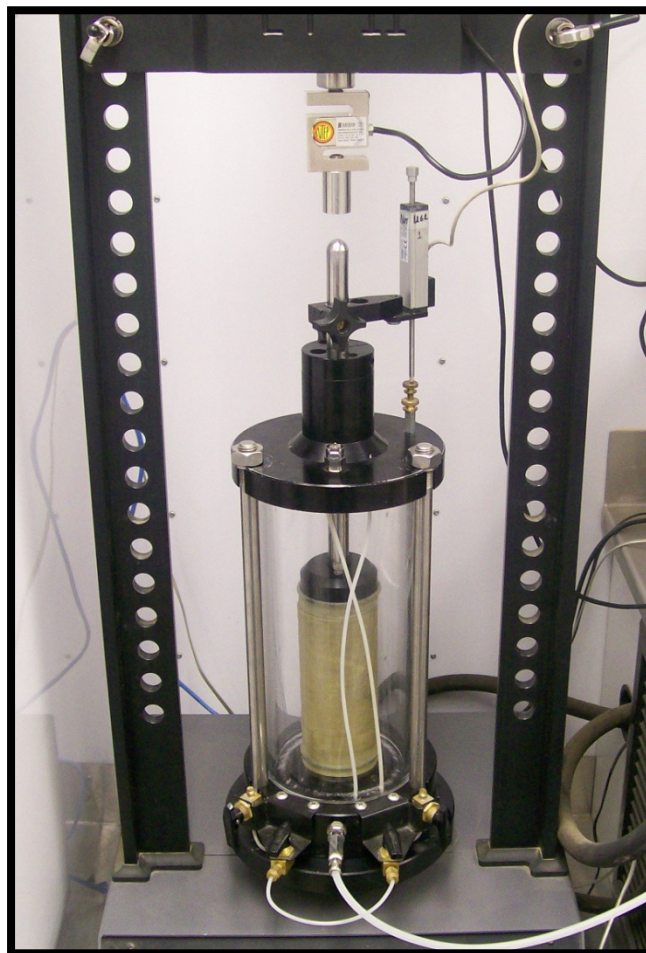
Figure 20: Actual Triaxial Chamber with External LVDT and Load Cell
